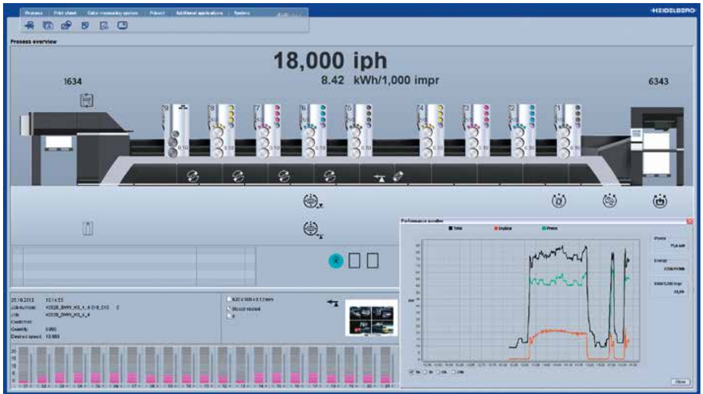
Prinetx Wallscreen: The energy efficiency value in kWh/1,000 sheets is displayed in real time.
