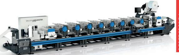
The Gallus Labelmaster Advanced line combines flexibility and cost-efficiency with the latest productivityboosting features: a digital printbar and front-loading rotary die-cutting.
