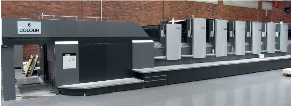
Freedom PrintPak's six-colour Heidelberg Speedmaster is placed in line with the company's new six-colour Speedmaster CD 102. The latter enables the doubling of sheet size to 720mm x 1 020mm and an increase of output to 15 000 sheets/hour.
