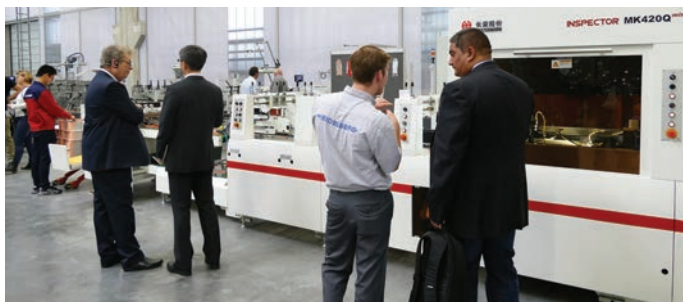
The MK Qmini 420/550 offline inspection system doesn't just check the print quality but also the embossing, foil and hologram positions, and the reverse of the sheet, thus ensuring the highest quality.
