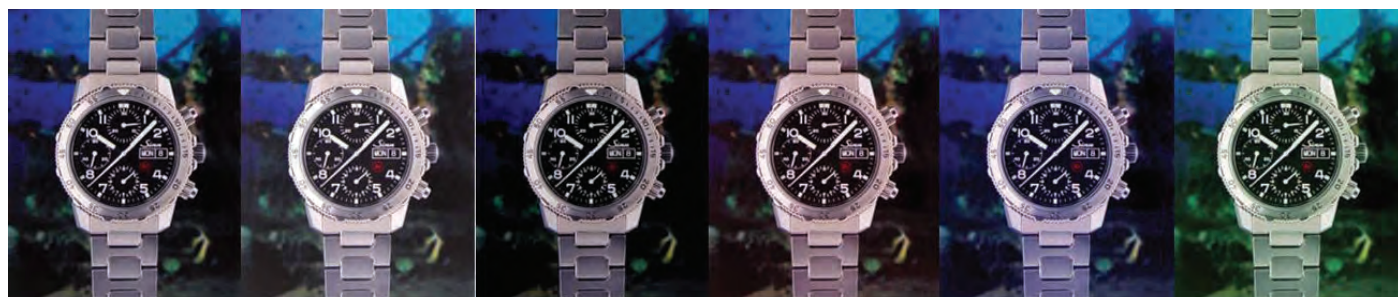
Above are examples of how mis-register can affect an image. The watch on the left is in register, the rest are not.
