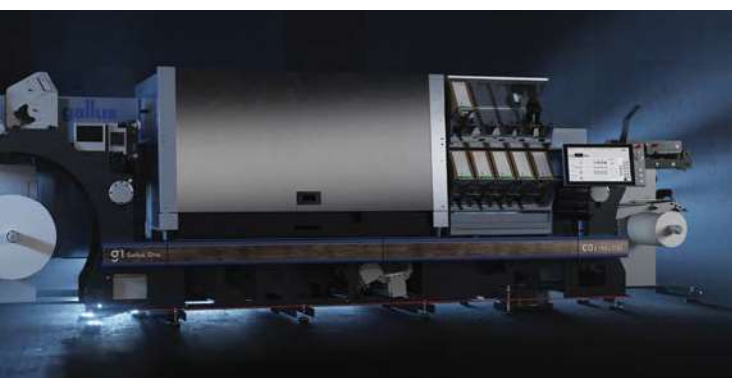
Renowned for achieving high levels of automation and press efficiency, the Gallus One boasts superior UV inkjet print quality and print speeds of up to 70m/min.
