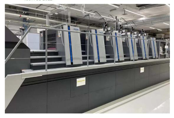
The Heidelberg Speedmaster XL 106 is a highly automated system from the 2020 generation with a Push to Stop configuration. Jobs that are added to the job queue are therefore completed automatically.
