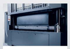
**Prinect Inspection Control 4** checks every sheet inline with high-resolution color cameras for errors before downstream costs are incurred.
