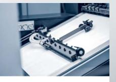
Antistatic equipment for metallized substrates and foils prevents the material from becoming charged.
