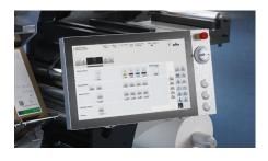
Human Machine Interface (HMI) is designed to summarize important information at a glance. For quality assurance, the print results can be checked live, via web video, or while the press is running.
