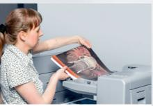
**Interposer** introduces pre-produced sheets into the pile during ongoing print production – for seamless inline postpress.
