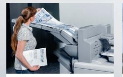
**Banner printing** up to 1,260 mm printed on one side or 1,030 mm printed on both sides. Suitable for the production of six to eight-pagers as well as large posters on one sheet.
