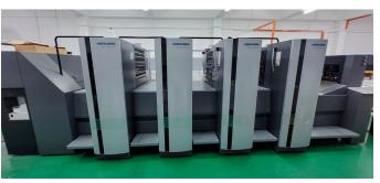
Make ready time, which previously took 30 minutes, have been significantly reduced to 15 minutes, while at the same time waste sheet has been cut by more than half. Production and output speeds have also increased by more than 50%, from 7,000 sheets to 11,000 sheets per hour, and a 20k job can be completed in less than two hours, including make ready. This has never been achieved before.
