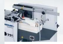
The **flat pile feeder** with sheet separator ensures safe sheet separation.
