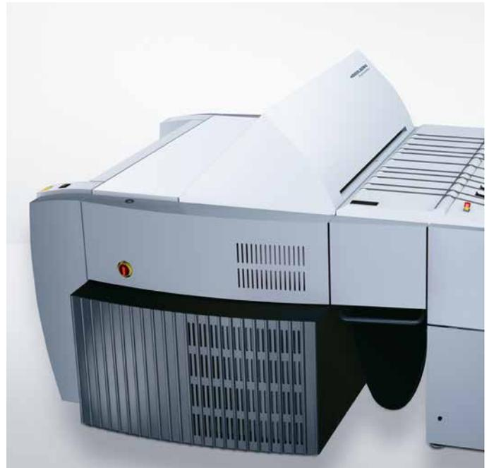
To make plate production even faster and ensure flexibility when using different plate formats, the Auto Pallet Loader can be used in parallel with the Auto Cassette Loader or the Dual Cassette Loader.
