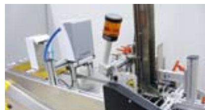
Personalized 360 dpi cards – the "FixedLine" drop-on-demand system developed in the Linoprint innovation project at Heidelberg.
