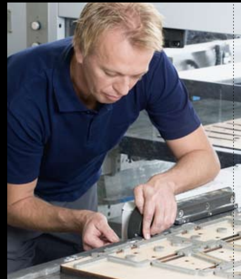
Øystein Hermansen (left) and Terje Holm prepare the Varimatrix 105 for die cutting and embossing the folding cartons.
