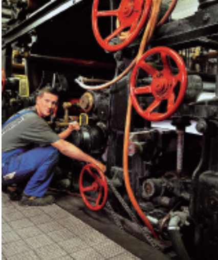
Employee Annika Peters with products made of Gmund papers. Cautiously, Nikolaus Weber drains the paper pulp with a 120 year old Fourdrinier machine. (from left)
