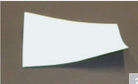
Raised corners on a paper test after storage in a warming cupboard.
