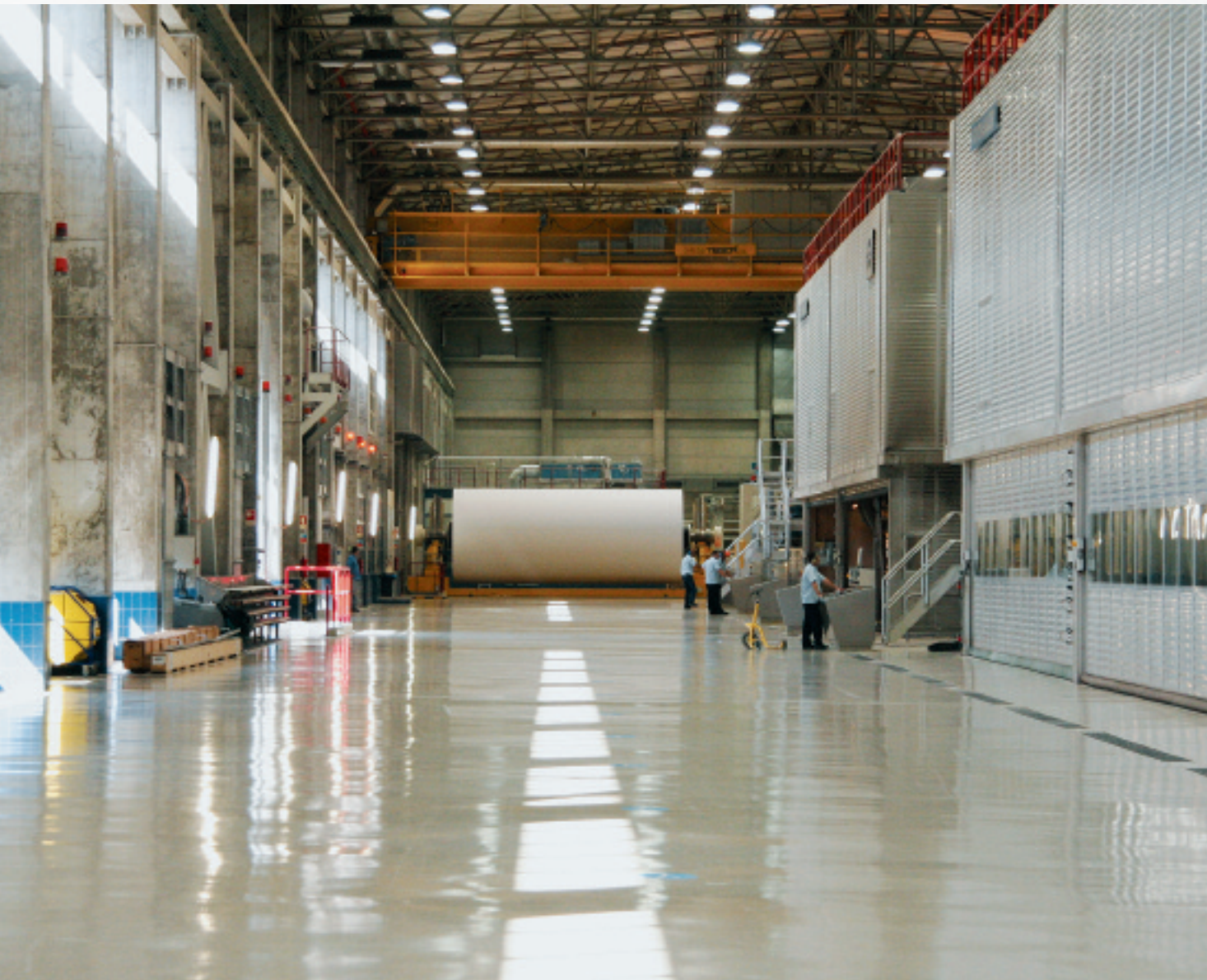
...with a total weight of as much as 50 tons by the end of the path. The 182 meter (600 ft.) long machine produces up to 1500 meters (5000 ft) of paper per minute. It is one of the two modern paper machines in Figueira da Foz.
