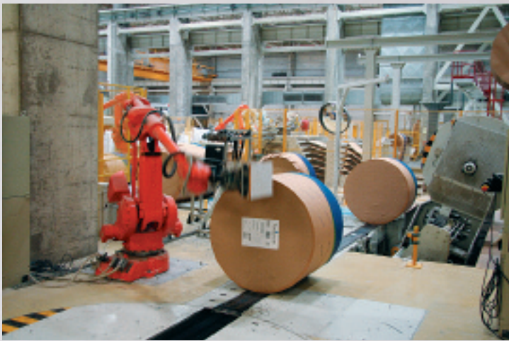
Fully automatic packaging: divided into “manageable” pieces, packaged and labeled, it is placed in high rack storage or shipped.
