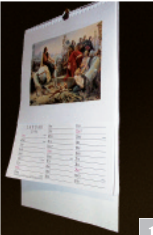
Raised corners on a rejected calendar.
