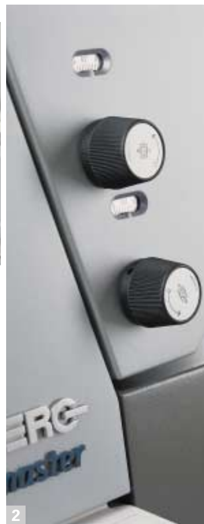
Simple register adjustment, even while the press is running.
