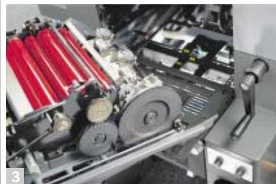
Numbering and stamping unit with integrated inking system.
