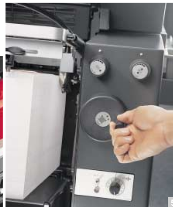
Central format adjustment for feeding and delivery unit.
