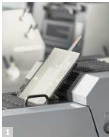
AutoPlate with integrated register system for both printing units.
