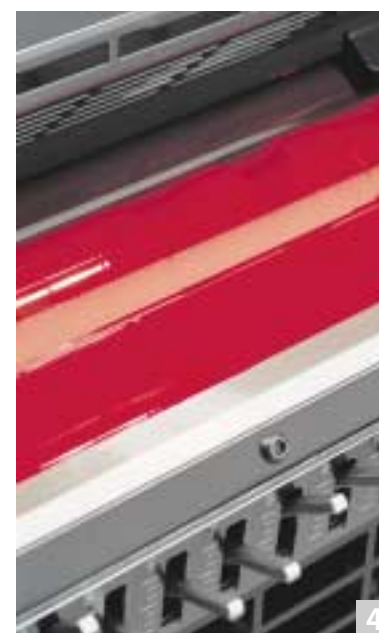
Laser-slit blade-type ink fountain with metering level.
