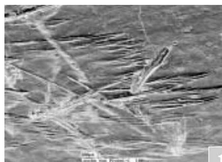
Damage to the cardboard surface from hard particles.
