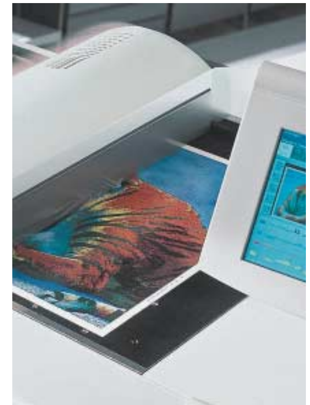
Prinect Image Control, a color measurement system used in quality control. It ensures print quality at a constant level.
