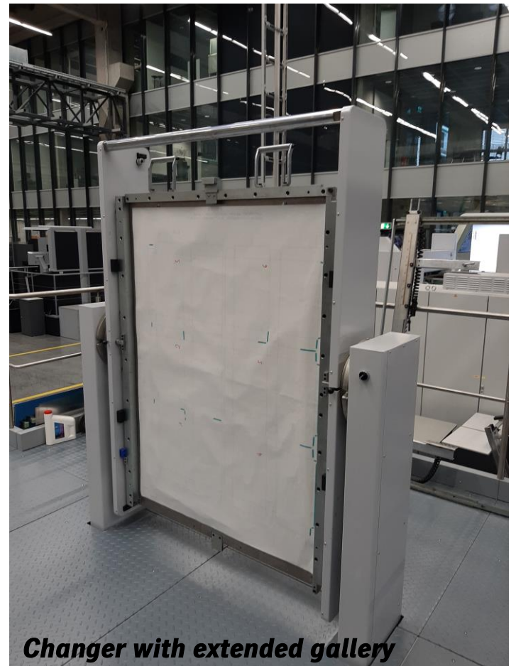
Auto-Non-Stop delivery with automatic pallet changer on top of the floor
