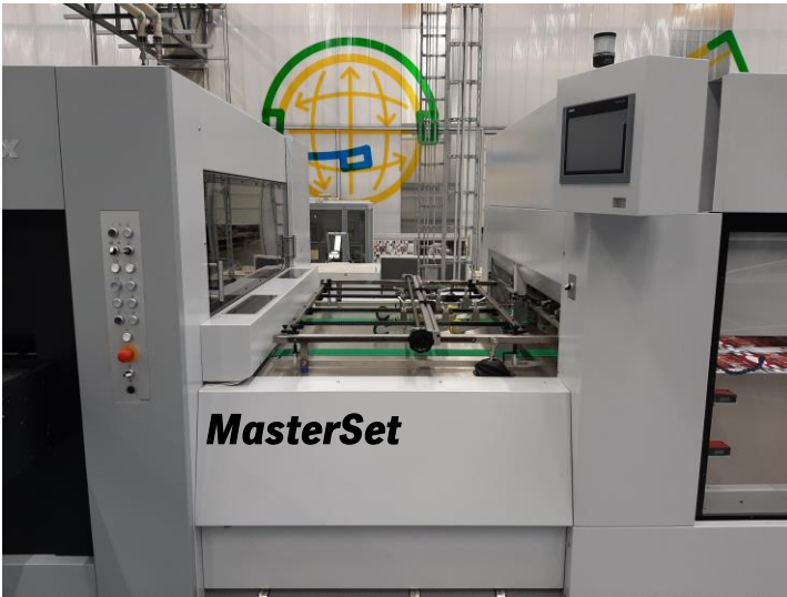
Auto-Non-Stop delivery with automatic pallet changer on top of the floor
