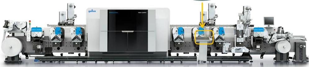
The DPU is perfectly integrated in the conventional machine. There is only one user panel to operate a Labelfire
