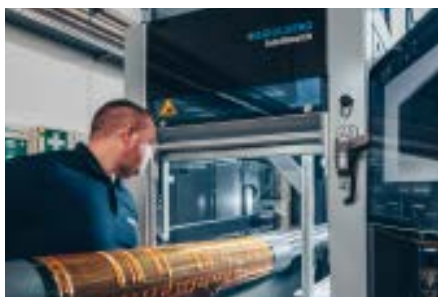
Intellimatch , the unique offline printing plate and sleeve scanner provides all press parameters for the Boardmaster.
