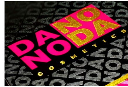
With screen printing you achieve outstanding haptic effects. The printing of security inks or micro particles like glitter is easily processable with screen printing.
