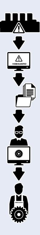
1. The Prinect Press Center transmits all key performance parameters over the Internet to the Heidelberg service center. 2. A service expert checks and evaluates data that gives cause for concern, such as voltage fluctuations or values close to specified limits.
