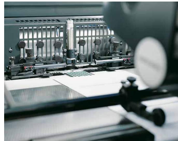
The suction tape feeder on the Printmaster PM 52 can be conveniently set up from the PressControl feeder panel.
