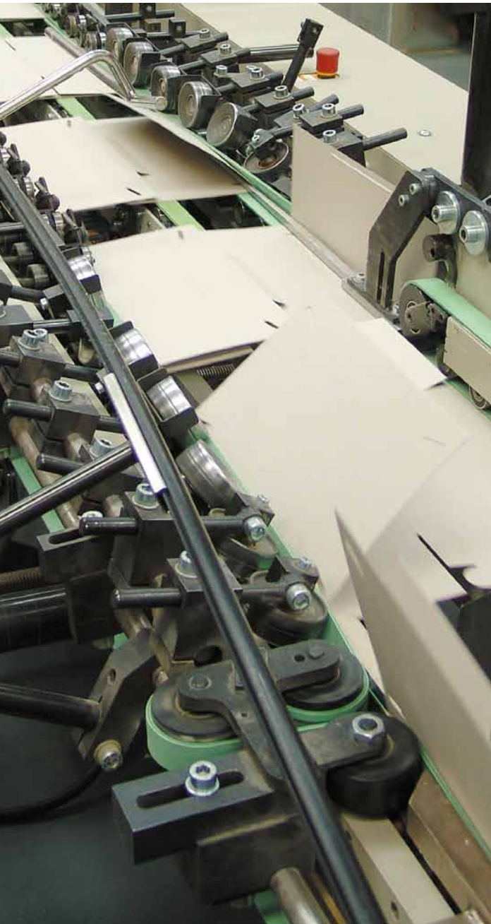
The Diana Pro features a highly versatile folding station and supports various different fold sequences.
