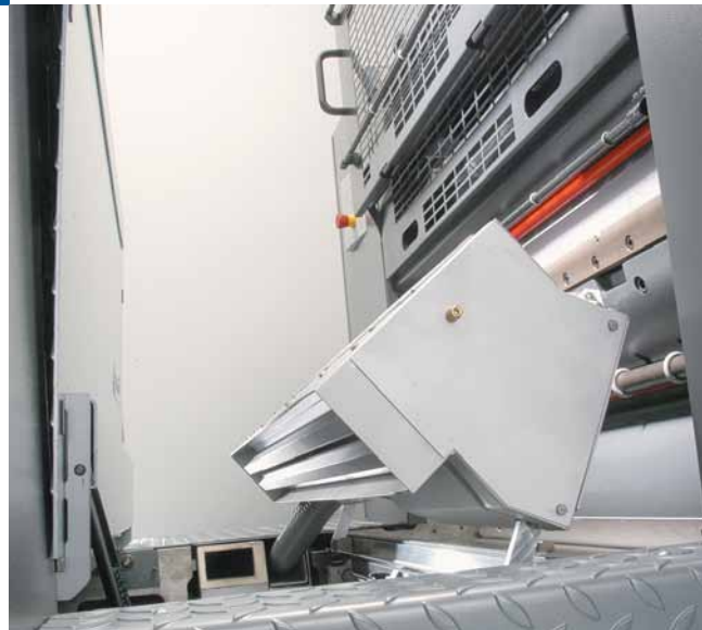
Interdeck dryer in swung-up position – the dryer can quickly and easily be moved between the individual printing units to the position required for each printing job.
