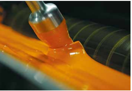
of which have a negative impact on production. Highly-viscous inks in the ink fountain are kept moving by InkMove.
