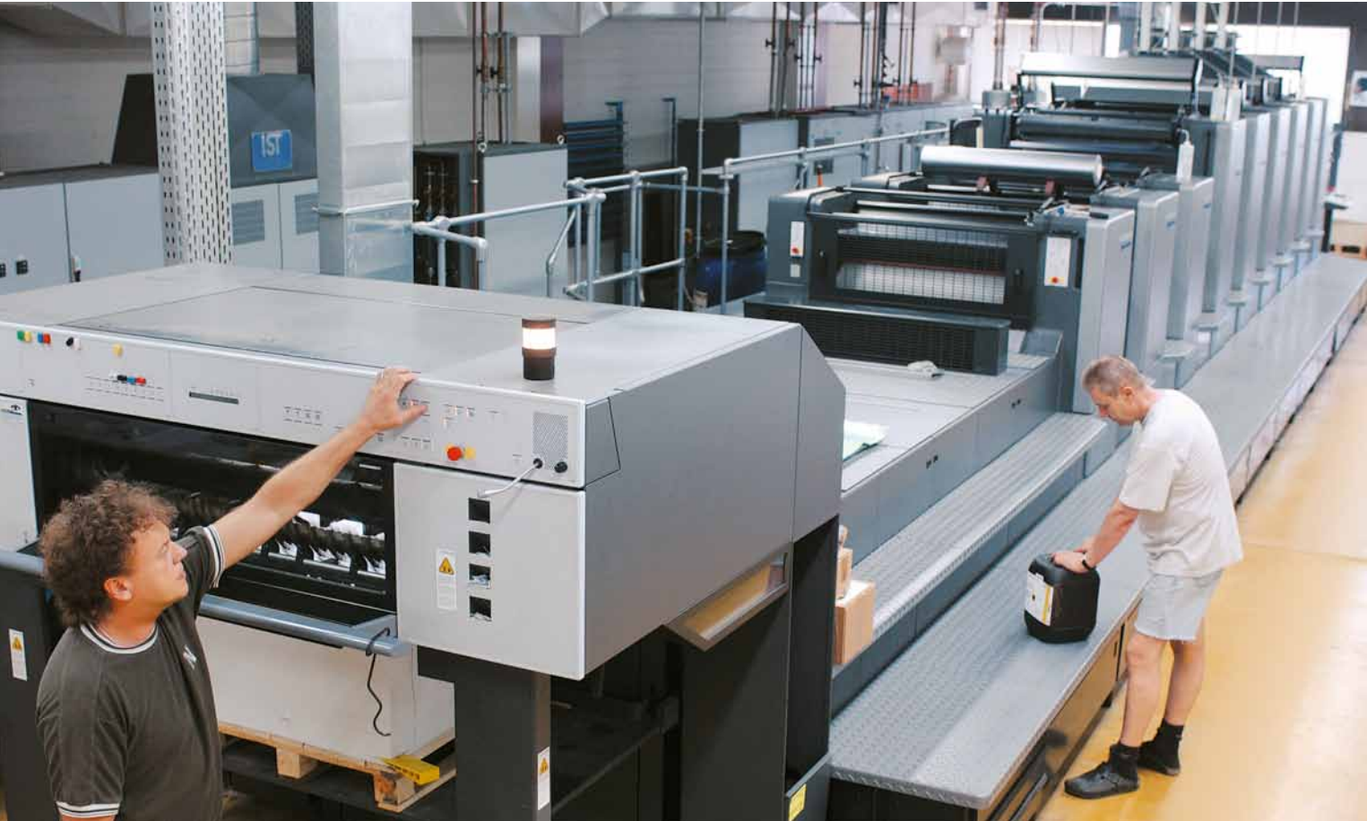
Olaf Herzog (front) and Michael Marquardt with the Speedmaster CD 102 at Multicolor in Ellerau. The dual coating press with extended delivery for inline UV coating features suction extraction of the ink mist above every inking unit.
