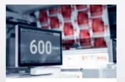
**High performance** with 600 m/min (2,000 fpm or 36,000 sheets per hour in format 7).
