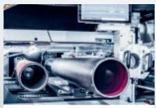
**Nonstop production** since one unit can be completely prepared for the next job while the other one is printing.
