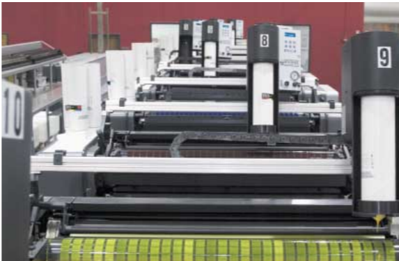
The new Speedmaster SM 102 has been equipped with an automatic ink refilling system.
