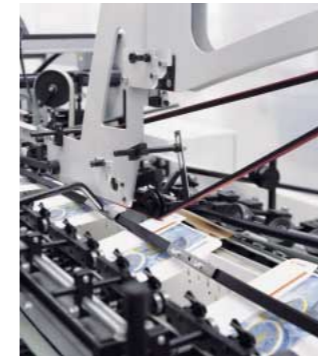
Separate servo-drives for each module give the Diana X flexible configuration options. The unit, which rotates the blanks and then aligns them correctly, allows 180 degree rotation. All control units are clearly structured and easy to understand. (left to right)
