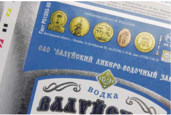
Typical Duo effect: Finest elements are printed on top of flexographic gold with offset colors (top). Opaque white over the flexographic unit produces high-ink coverage, also on metallized materials (bottom).
