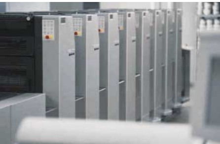
The eight-color Speedmaster SM 52 with sheet reversal, ideal for 4/4 jobs or laying down up to eight colors on one side of the sheet.
