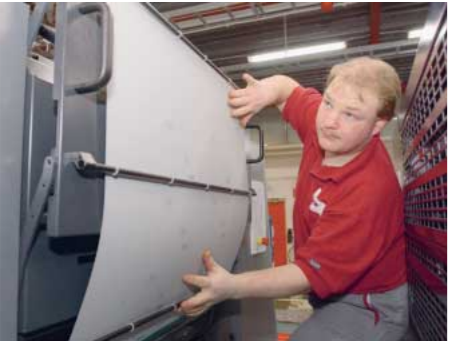
Plate changing on the Speedmaster CD 74.
