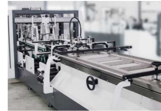
Separate servo-drives for each module give the Diana X flexible configuration options. The unit, which rotates the blanks and then aligns them correctly, allows 180 degree rotation. All control units are clearly structured and easy to understand. (left to right)
