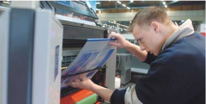
Benjamin Balasunderam of Germany mounting a fresh printing plate. Jordan Poulain from Belgium replenishing the ink. (Left to right)
