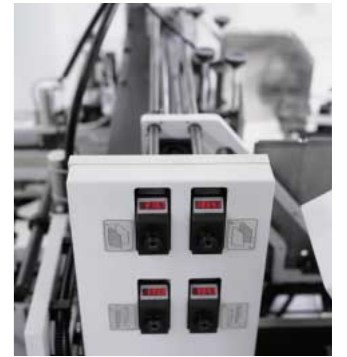
Separate servo-drives for each module give the Diana X flexible configuration options. The unit, which rotates the blanks and then aligns them correctly, allows 180 degree rotation. All control units are clearly structured and easy to understand. (left to right)
