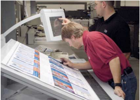
Printers Cary Lumsden and Bradley Pfeil checking print sheets and setting up the presses using the Prinect CP2000 Center (left to right).
