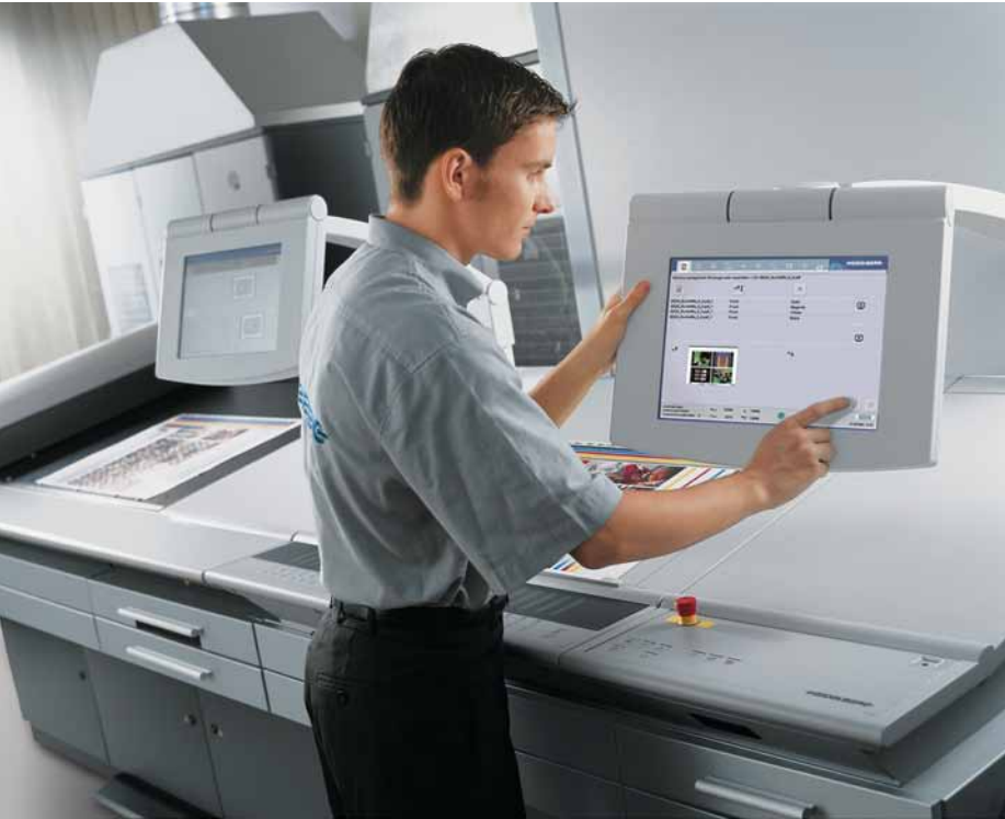
The Prinect CP2000 Center press control system provides access to all job data required for plate imaging. The plate-on-demand function is quick and easy to use by touchscreen.
