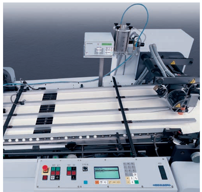
Intermittent glue lines, variable spot gaps and sizes, and in-plate cold glue guns for auxiliary gluing without segmenting the folding rollers.
