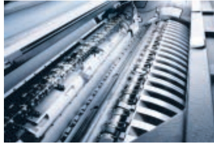
Perfecting device with fully automatic adjustment for precise registration, even at top speeds.
