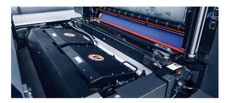
The integrated Prinect Inspection Control 4 inline sheet inspection system reliably detects the smallest print and material defects. For this purpose, printed sheets are permanently compared with a digital reference value. The optimal sheet guidance enables comprehensive inspection up to the rear edge of the sheet.
