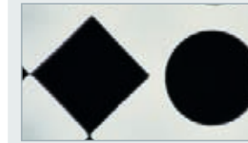
Two halftone dots on film (magnified approx. 150x)
