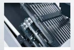
The **motorized combination buckle plates** enable precise positioning of the sheet stop.
