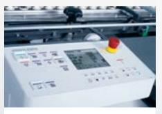
The **control panel MCT** ensures quick intervention through control panels at the feeder and the subsequent stations.
