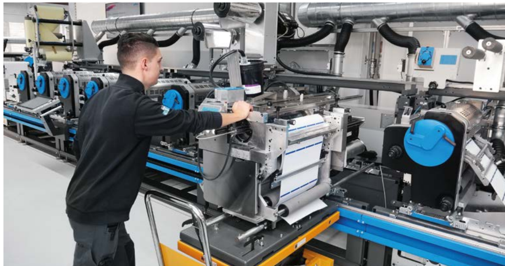
The different printing processes can be changed at any position of the machine.
