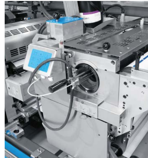
The screen printing unit can be positioned on any module of the Gallus Labelmaster and thus becomes a fully integrated component of the machine system.
