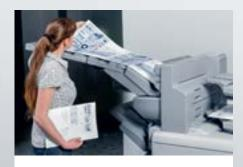
**Banner printing** up to 1,260 mm printed on one side or 1,030 mm printed on both sides. Suitable for the production of six to eight-pagers as well as large posters on one sheet.
