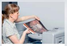
**Interposer** introduces pre-produced sheets into the pile during ongoing print production – for seamless inline postpress.
