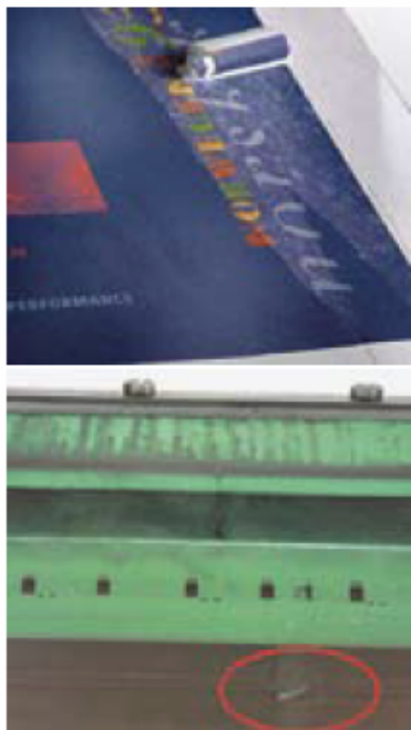
Layers can roll up in the pile up to 15 times during various motion processes. This leads to rolled-up strips on the printing stock. If these are run through the printing press, the printing blankets inevitably get damaged and in extreme cases, other units can also be damaged.
