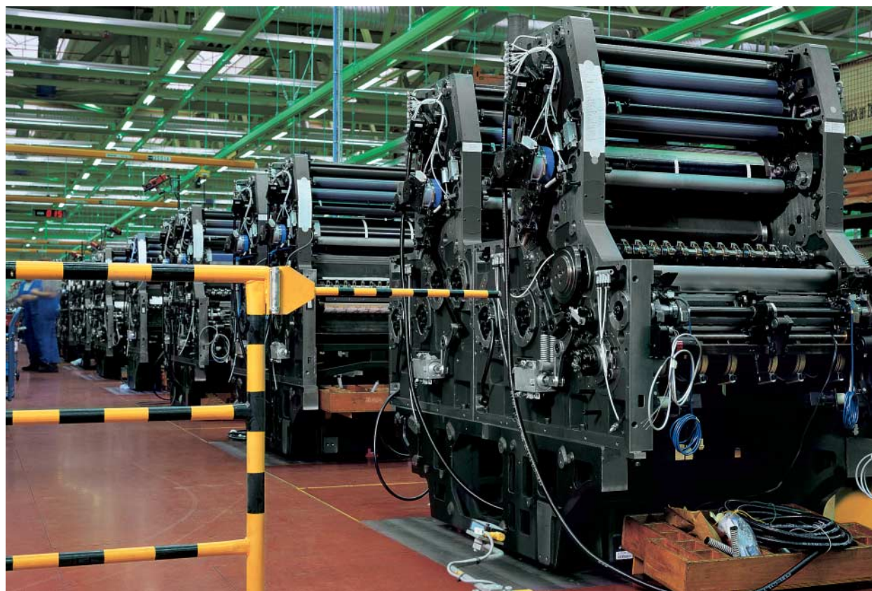
Assembly in the Wiesloch works: printing units of the Speedmaster series are assembled as they pass through the hall. For more than 20 years the Speedmaster has been one of the company's most successful product lines.
