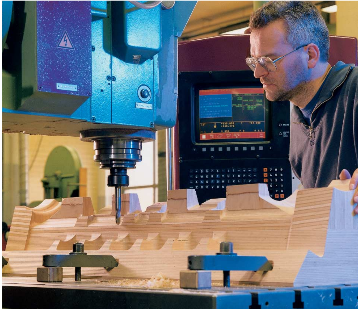
Mold production in Amstetten: the foundry produces blanks for all of the iron casting parts of Heidelberg offset presses.
