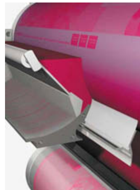
The ink chamber blade system, made with an ink chamber and a doctor blade, fills the screen roller with ink.
