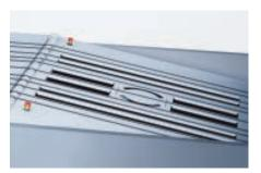
The Dual Cassette Loader (DCL) with integrated turn table automates the loading of plates into the Suprasetter.
