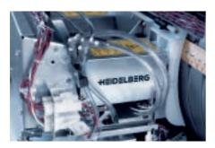
The laser module offers outstanding quality and a high level of reliability thanks to the patented Intelligent Diode System (IDS).
