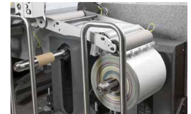
The double rewinder* enables crossed winding of rolls. * contains optional equipment
