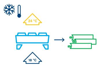
For temperatures up to 20 °C (68 °F), the inking unit is cooled using free cooling, i.e. via the recooler of the water cooling.
