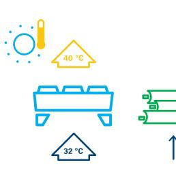
Free cooling is not used for temperatures above 20 °C (68 °F) and the inking unit is cooled conventionally using refrigeration compressors.
