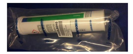
\* Saphira multi temp grease used for lubricating all Cam followers and Gripper bars
