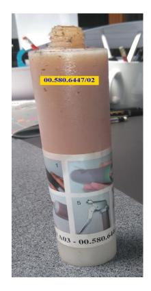
\* Saphira multi temp grease used for lubricating all Cam followers and Gripper bars
