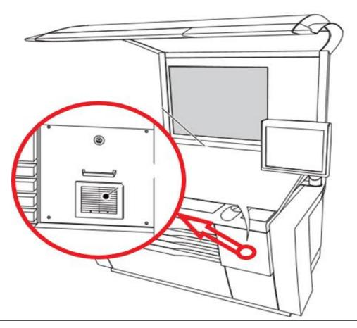
\* Filter for Inpress Control located on the left-hand side of the consol
